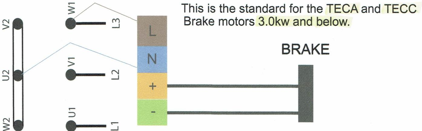
Brake can also be separately supplied. Motors with a Star/Delta starter must have a separate supply to the brake.
