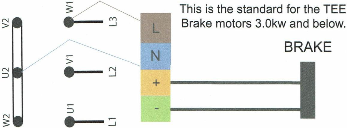
1/2 Wave 178V/190V brake. Phase and Phase connection
