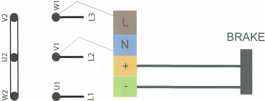
Full Wave 178v/190v brake. Phase and Star point connection
