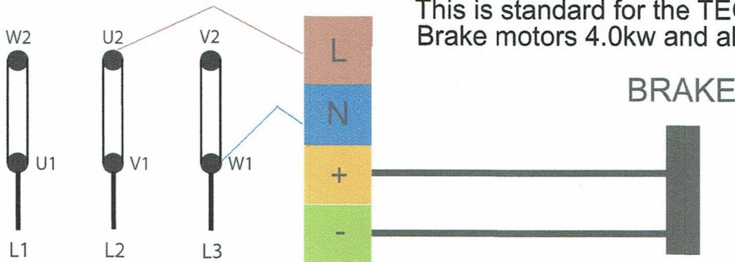
Full Wave 178V/190V brake. Phase from motor and separate neutral
