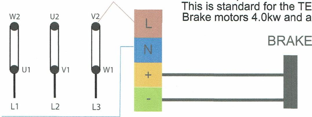
1/2 Wave 178V/190V brake. Phase and phase connections
