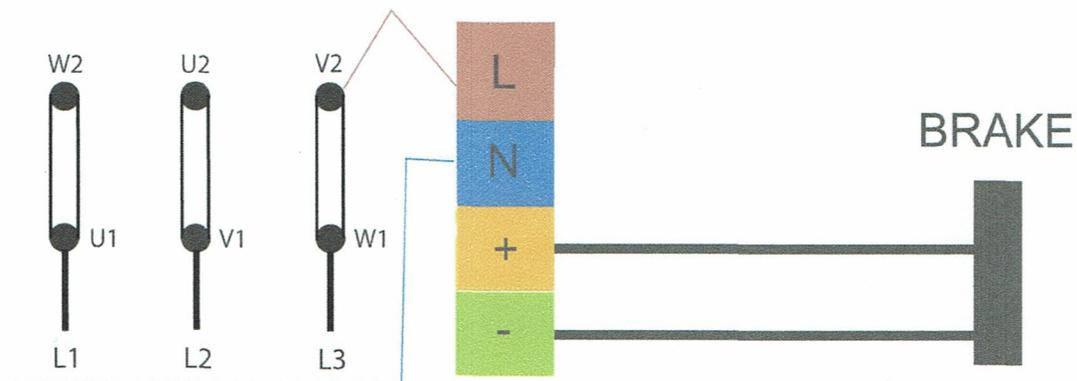
Brake can also be separately supplied. Motors with a Star/Delta starter must have a separate supply to the brake.
