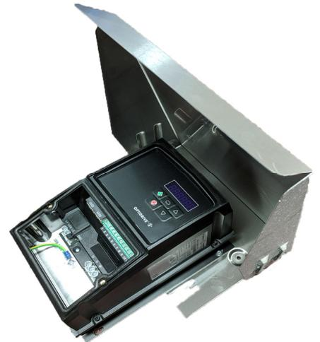
**Step 4:** Connect the other end of the earth lead to the inverter's earth terminal as shown below, or to another suitable earth connection point.
