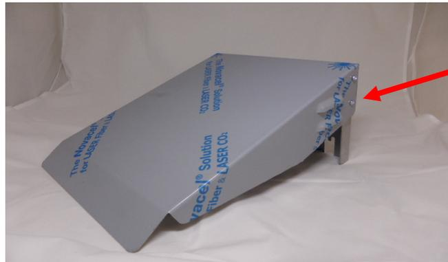
**Step 1:** After removing the plastic covering, fix the two sections of the cover together using the 4 off M4x12 bolts with 1x flat washer , 1x spring washer and 1x M4 nut (supplied) making sure that the supplied earth cable is fitted to the left hand bottom bolt as shown below.
