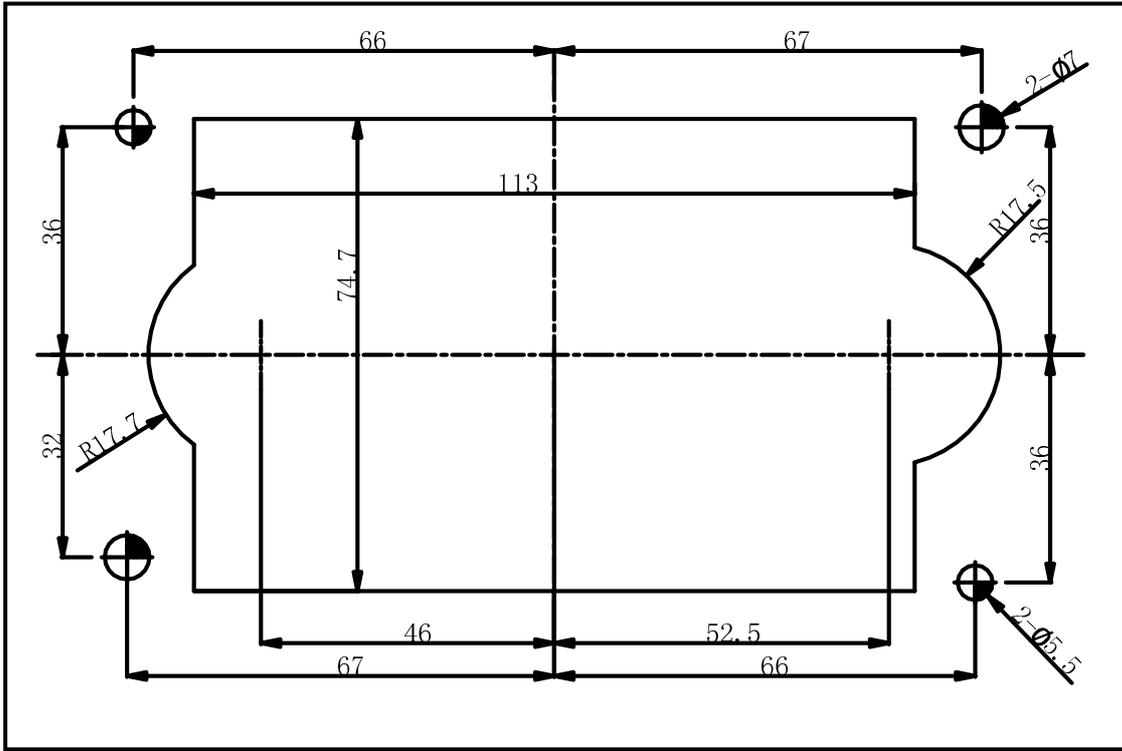
In order to reduce the difficulty of the keypad installation, the mounting dimensions as shown below are recommended:
